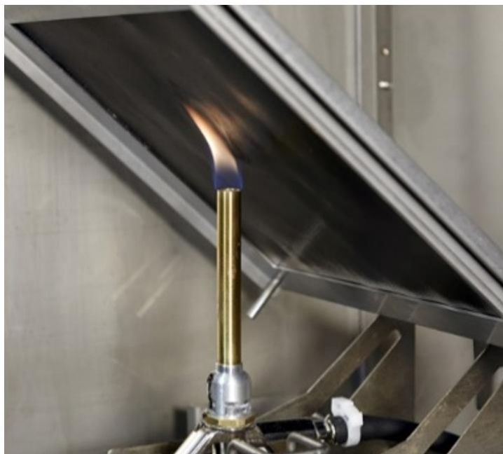
Figure 3. Typical 45° burning arrangement.
