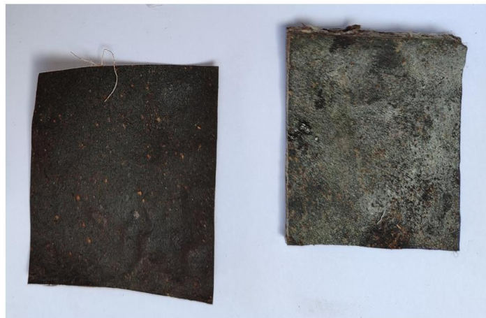
Figure 4. Banana peel-treated bio-coated fabric and banana peel-associated bio-composite from left to right.
